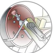
Gas striker for remote operation of the hydraulic opening valve
