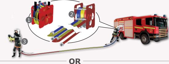
1 - Connect the hoses together, one end will be connected to the water inlet, the other to the hand nozzle.
