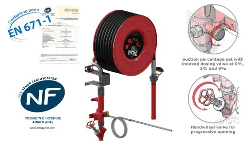
The new FHR (Foam Hose Reel) POK, DN33, swivelling-rotating, is conform to norm EN 671-1 and is also certified by AFNOR. Entirely developed by POK, it benefits from our great know-how in the creation of foam products. Its eductor is adjustable in 3 positions: 0%, 3%, 6 %, in order to obtain a quality low expansion foam.
