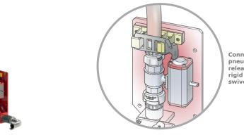
Connecting plate with pneumatic valve, quickrelease coupling, semirigid connecting hose, and swivelling outlet elbow
